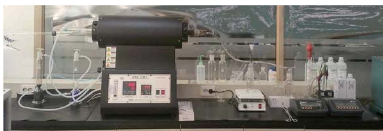
Cable Gas Tester IEC 60754-1 / IEC 60754-2
