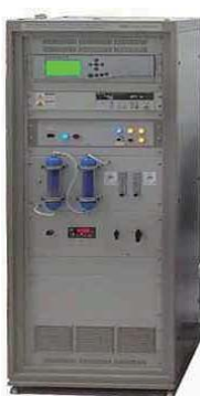
Gas extraction analysis rack
