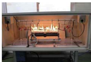
IEC 60331 or BS 6387 Fire Resistance Test
