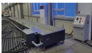
35m water bath for High voltage test in water
