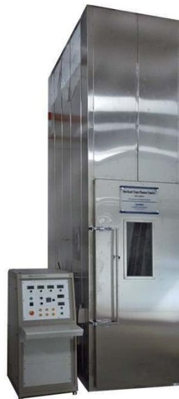
Vertical Flame Resistance Tester IEC 60331-3-10 IEC 60331-3-22
